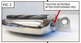
**WARNING** FOOTPEGS MUST BE INSTALLED SO THEY WILL FOLD UPWARD AND REARWARD IF HIT BY ANY OBJECT. FAILURE TO ADJUST THE FOOTPEGS TO OPERATE IN THIS MANNER COULD RESULT IN SERIOUS INJURY OR DEATH.
