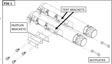
Using the included  $5/16''-18 \times 3/4''$  hex head bolts, nuts, and washers, attach the muffler bracket to the support bracket; leave them loose at this time.
