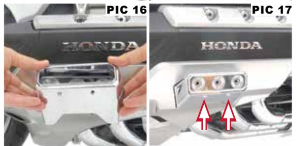
**STEP 15** Refer to PIC 16 and 17. Locate provided Left Mount Cover. Align and place it over the casting and bracket assembly and into the Cylinder Head Side Cover.
