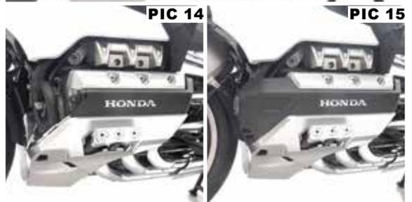
**STEP 14** Refer to PIC 15. Locate the Fog Light Cover and mounting hardware that was removed in Step 3. Align and fasten the cover to the motorcycle. Fully tighten all hardware.
