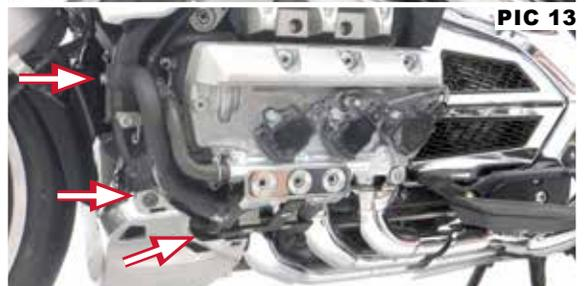
**STEP 11** Tighten all flat head screws located on the bottom of the bracket that is fastened to the casting piece.
