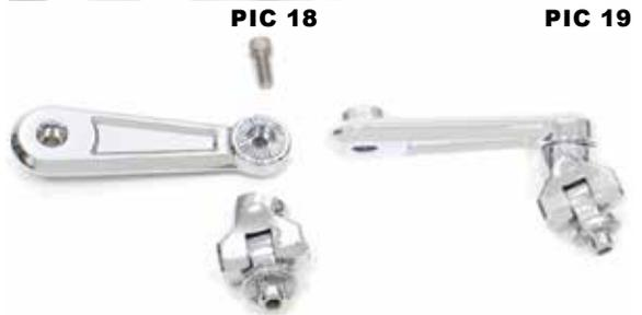
**STEP 17** Refer to PIC 18 and 19. Locate provided Left Clevis (clevis bends back towards the rear of the bike and the set screw is located on the bottom side), one (1) pivot arm and one (1) 5/16-18 X .75 Socket Head Cap Screw. Apply a small amount of blue Loctite to the threads of the screw. Align the splines of the clevis and the top of the pivot arm. Secure the clevis to the pivot arm by inserting the screw from the backside of the pivot arm. Do not fully tighten the hardware yet.
