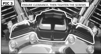
STEP 6 Torque the two lifter cover screws to 90-120 inlbs (10.2-13.6 Nm).
