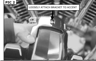
STEP 4 Refer to PIC 3. Hold the Accent in place, then thread the two screws through the Bracket and into the lifter covers; leave them loose for now to allow for adjustment.
