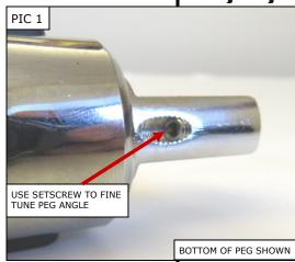
FOOTPEGS MUST BE INSTALLED SO THEY WILL FOLD UPWARD AND WARNING REARWARD IF HIT BY ANY OBJECT. FAILURE TO ADJUST THE FOOTPEGS TO OPERATE IN THIS MANNER COULD RESULT IN SERIOUS INJURY OR DEATH.
