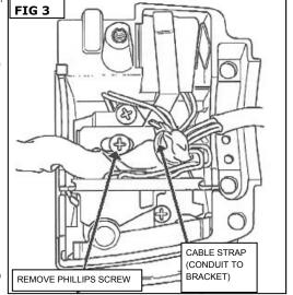
STEP 12 Disassemble the right lower switch housing. See FIG.3. Carefully cut the cable strap holding the wire conduit to the turn signal switch bracket.
