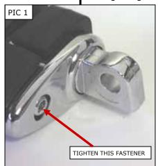
FOOTPEGS MUST BE INSTALLED SO THEY WILL FOLD UPWARD AND WARNING REARWARD IF HIT BY ANY OBJECT. FAILURE TO ADJUST THE FOOTPEGS TO OPERATE IN THIS MANNER COULD RESULT IN SERIOUS INJURY OR DEATH.
