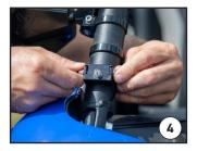
1. Remove the thumb screws, rubber washers, and nylon washers from the assembled kits. 2. Clamp instructions are provided on the back of the red card. 3. Install one clamp on each side of the front roll bars. 4. Install Axia insert and finger tighten clamp bolts.
