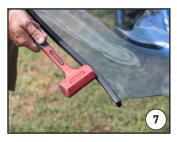
**5.** Place black plastic washers on both studs. **6.** A single piece of trim has been supplied to cover the bottom of the Flare™ Windshield. **7.** With the bulb facing the back side of the windshield, install trim on the lower lip. A rubber mallet may be needed to fully seat the trim (**BE GENTLE**).
