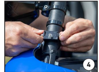
1. Remove the thumb screws, rubber washers, and nylon washers from the assembled kits. 2. Clamp instructions are provided on the back of the red card. 3. Install one clamp on each side of the front roll bars. 4. Install Axia insert and finger tighten clamp bolts.
