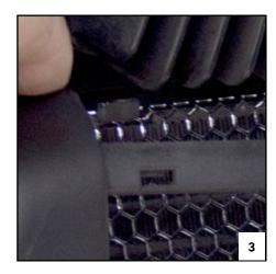
1. Remove the oil cooler cover by pulling the two lower pins from the rubber grommets on the cooler and rotate forward to allow the top to be released from tabs (FIG 1).
