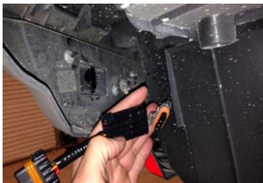
1. Simply unplug the stock harness plug from the back side of the factory tail light.
