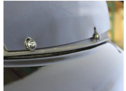
3. Install your new Flare™ Windshield onto the mounting screws and torque to factory specifications
