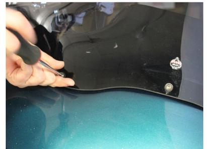
3. Starting with the center screw, install your new Flare™ Windshield and torque to factory specifications.
