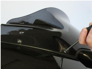
1. Loosen, but do not remove, the four windshield mounting screws and gently remove your windshield
