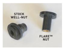
2. Check the well-nuts in the fairing, if they are damaged or broken, Klock Werks offers a replacement kit (part number 2404-0548) for \$29.95
