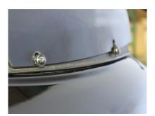
3. Install your new Flare™ Windshield onto the mounting screws and torque to factory specifications
