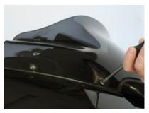
1. Loosen, but do not remove, the four windshield mounting screws and gently remove your windshield
