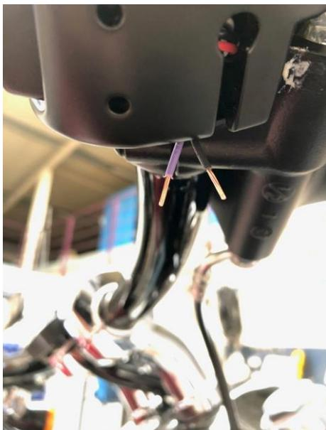
5. Install the Kodlin turn signals and trim the cable to the right size (about 4" long)
