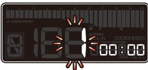
● In the clock setting screen, hold the **button for 3 seconds** to enter into the set up screen.
