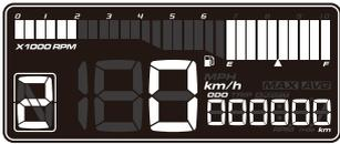
•In the total mileage screen, press the **button once** to switch to Trip A screen.
