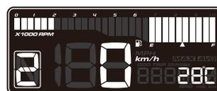
•In the engine temperature screen, press the **button once** to switch to the voltage screen.
