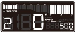
•In the mileage maintenance screen, press the **button once** to switch to the remaining mileage screen.
