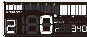
•In the remaining mileage screen, press the **button once** to switch to the average fuel consumption screen.
