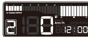
•In the clock screen, press the **button once** to switch to the engine temperature screen.
