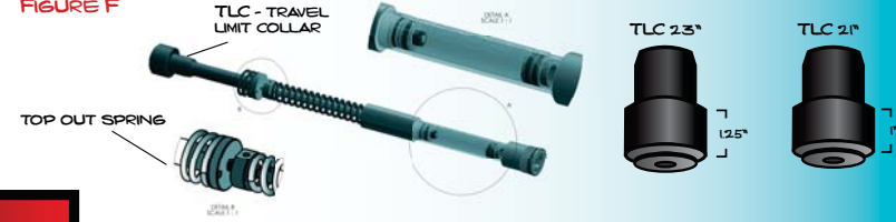
FIGURE E (TLC - TRAVEL LIMIT COLLAR)
