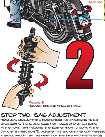
OVER BUMPS THERE ARE ALSO POT HOLES AND OTHER GAPS IN THE ROAD THAT REQUIRE THE SUSPENSION TO WORK IN THE OPPOSITE DIRECTION. TO ACHIEVE THIS SHOCKS ARE COMPRESSED A SMALL AMOUNT BY THE WEIGHT OF THE BIKE AND THE RIDER(S). THIS IS CALLED SAG AND IS ADJUSTED BY PRE LOADING THE SPRING AS SHOWN IN FIGURE B.
