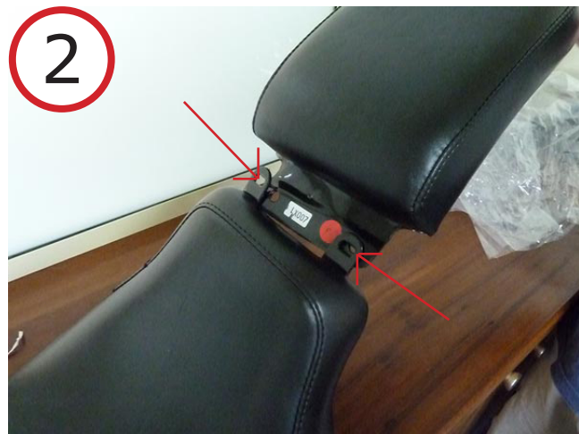
Tags on Rider Seat are no longer used to mount the seat
