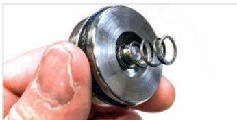
*If you have a Milwaukee Eight model, you must also put the clutch sleeve onto the piston.*
