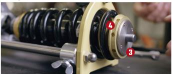
**8.** The height of the bike will be adjusted with the spring washer (Pos. 3). For a maximum lowering of 40mm you must rotate the spring washer (Pos. 3) all the way onto the damper rod.
