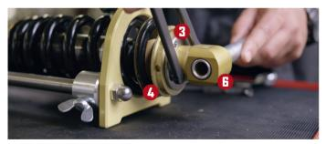
**11.** Use a C-spanner for adjusting the chassis curing and preload the spring with a spring compressor (Pos. **4**). The chassis curing can be re-adjusted any time.
