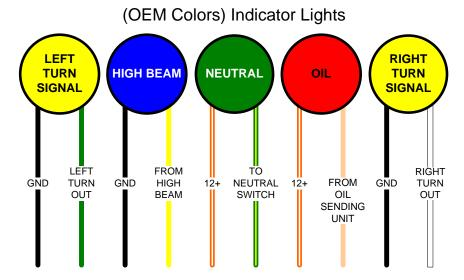
When wiring the indicator lights, be sure to twist ALL (3) of the black wires together and BOTH (2) of the orange/white wires together when attaching to our harness.
