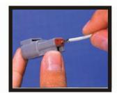
3. Push contact straight into the connector grommet until a "click" is felt. A slight tug will confirm that it is properly locked in place
