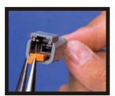
1. Remove orange wedge using needle nose pliers to wedge straight out.
