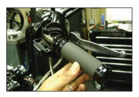
4. Position upper and lower switch housings on handlebar. Tighten two screws to factory torque specs. Make sure throttle works smoothly! (you may need to adjust brake lever mount location)
