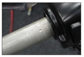
6. Use red Loctite and the supplied 5/64 ALLEN, tighten two screws on the grip. Make sure grip secure.
