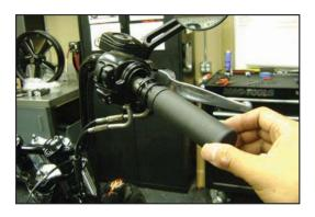
3. Slide throttle grip onto handlebar and insert cable ends into grip.
