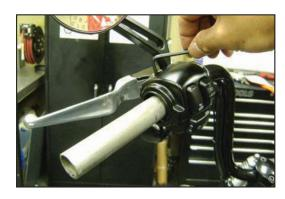
4. Slide on new left side grip until the grip stops against switch housing. Look at the end of the grip to position the logo where you prefer then mark the set screw locations through the threaded holes using a transfer punch and a hammer.
