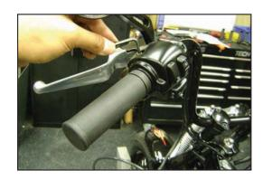
2. Use long flathead screw driver, brake loose adhesive between grip and handlebar otherwise use a sharp blade to carefully cut rubber grip off.
