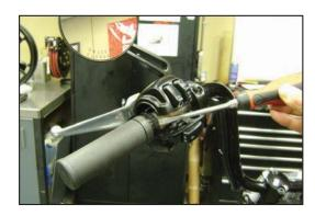
3. Install left side upper and lower switch housing on handle bar. Tighten two T25 TORX screws to factory torque specs.
