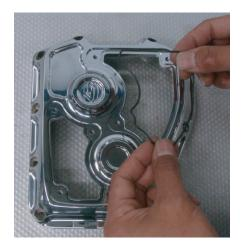
6. Peal the protective paper from the new clarity window(s). Clean using Plexus if necessary and place onto the cover. Install the supplied bolts with pre-applied thread locking compound. Do not torque the bolts until all bolts are installed.
