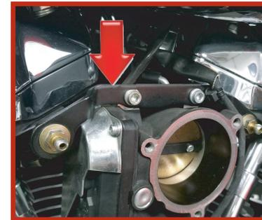
3. Install the backing plate using the supplied breather bolts, standoffs, throttle body bolts, spacer and gasket. Torque the 1/4-20 bolts to 8-ft lb and the breather bolts to 15 ft-lbs
