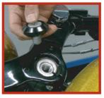
4. Install the Misano washer and bolt.
