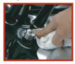
Install the Misano top nut and torque to 40 ft-lbs.
