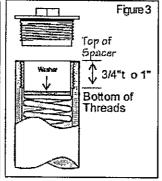
Also check the Notes in the enclosed Application Supplement, the stock spacer in some cases can be modified to fit. If making a spacer, we recommend PVC pipe that is the approximate diameter of the fork springs but will still fit inside the fork tubes. Warning:
