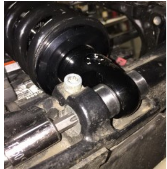
Wide Bearing Spacers with O-Rings installed as shown and installed at rear shock mount (swingarm).
