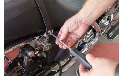
2. Pull seat strap to one side and remove seat.
