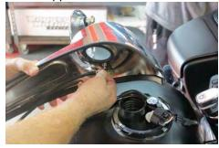
6. Pull overflow hose up from inside the chassis and discard.
