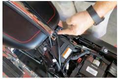
10. Install mounting screws, just finger tight for now. We will tighten them in a later step.
