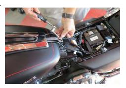
5. Carefully lift dash and bend back the retainer tabs to release the vent and overflow hoses. Disconnect the overflow hose from the overflow nipple.
