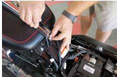
11. Install the fuel cap. Center the dash on the fuel cap and tighten the mounting screws. Use stock cap gasket if necessary.
