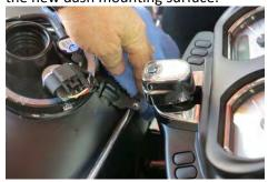
8. Install rubber trim moulding around the edge of the new dash, using masking tape to temporarily hold it in place. Make a small slit in the front with a razor blade to allow the rubber to follow the contour of the front of the dash. Apply CA glue in several spots around the moulding on the inside surface of the dash.
