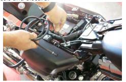
7. Using a towel to protect the paint, gently pry the mounting tab up slightly to match the angle of the new dash mounting surface.
