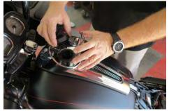
4. Remove front and rear mounting screws.
