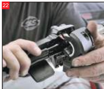
22 Reinstall the switch housings loosely around the switches.
