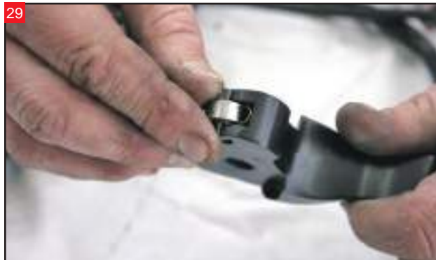
29 The small bearing from the stock lever is also reused in the new Racing Lever.
