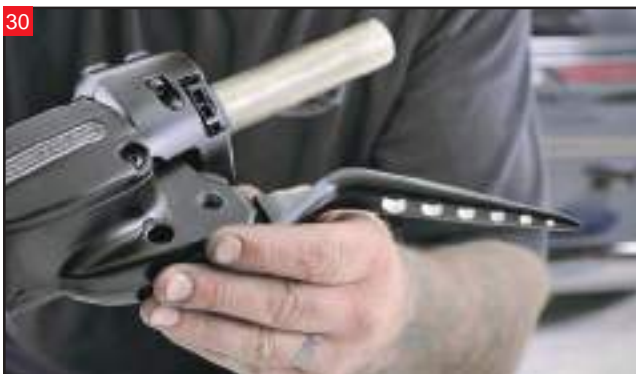
30 Position the Bagger Nation lever in the clutch perch.
