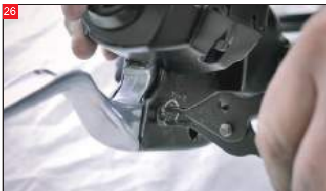
26 Remove the retaining ring from the pivot pin for the clutch lever.
