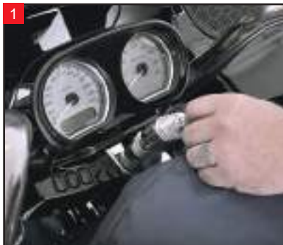
1 Place the key in the ignition switch. Mash the detent at the bottom of the switch while turning the key counter-clockwise. The ignition switch will lift up and out of the ignition post.
