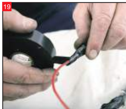
19 Attach the end of the switch housing wiring to the weed eater line using electrical tape.
