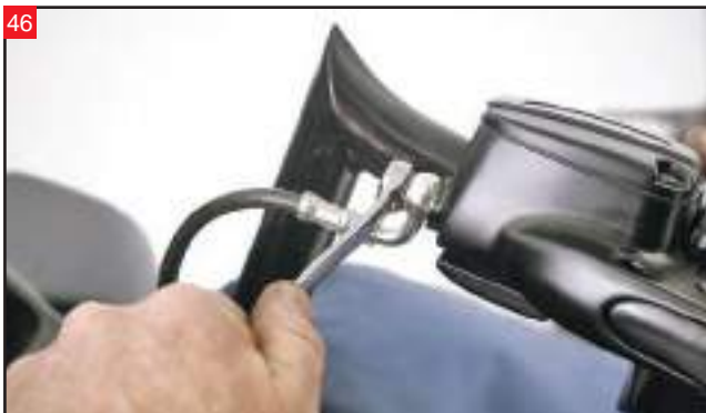
Tighten the banjo bolts with a 12mm wrench. Be sure to bleed the clutch and front brake if necessary.
