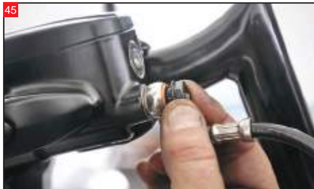
Reconnect the lines for the front brake and clutch master cylinder. Use new crush washers when installing the banjo bolts.
