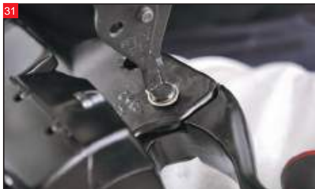
31 Reinstall the pivot pin with retaining ring.
