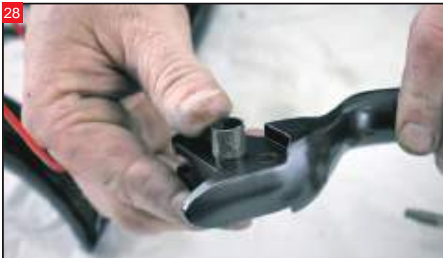
28 Install the nylon bushing from the stock lever into the Bagger Nation Racing Lever.
