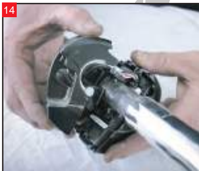
14 Remove the switch housing from the handlebars.
