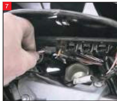
7 Unplug the connector for the TGS (Twist Grip Sensor).
