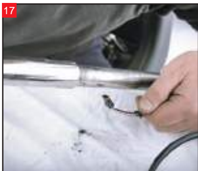
17 Remove the wiring from the inside of the stock handlebars.
