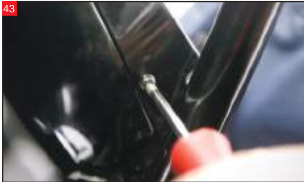
Install the housing over the nacelle with the two screws, one for each side. Tighten the screws with a T25 Torx.
