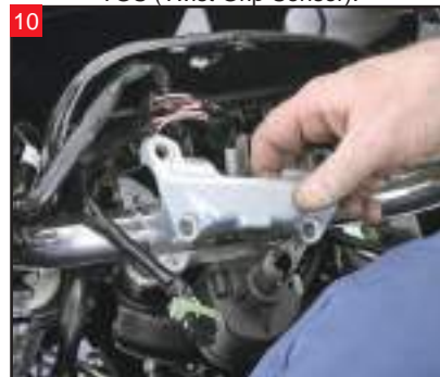
10 Remove the top clamp from the handlebar risers.
