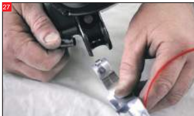
27 Lift the pivot pin from the housing to free the clutch lever.
