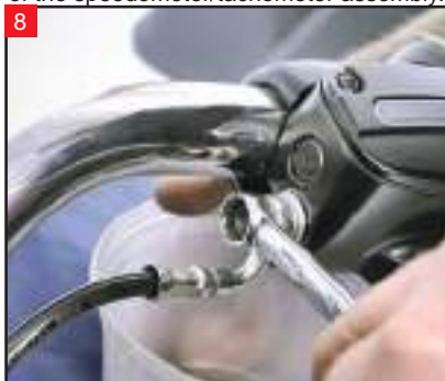
8 With a 12mm wrench, remove the banjo bolts at the clutch and front brake master cylinder. Have a small container ready to catch any brake fluid that may leak out. With the hydraulic lines free, reinstall the banjo bolts with a short section of 3/8" hose.
