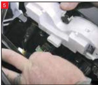
5 Unplug the single connector on the back of the speedometer/tachometer assembly.
