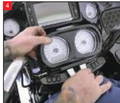
4 Lift the housing off the nacelle to access the wiring connectors inside.
