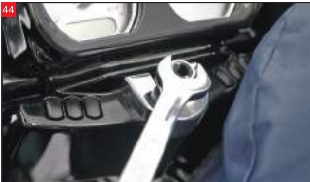
After installing the plastic spacers over the ignition post, tighten the top nut with a 7/8" wrench.
