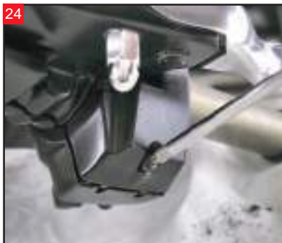
24 Tighten the hardware for the master cylinder and switch housing with Torx drivers.
