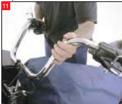
11 Lift the stock handlebars up and off the risers. Ensure all internal wiring is clear of the speedometer/tachometer nacelle.
