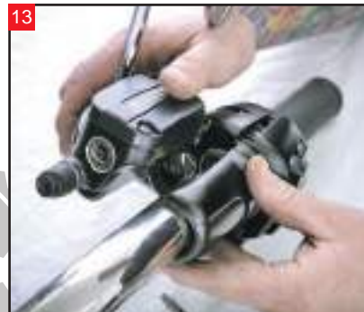
13 With a T27 Torx, remove the bolts holding the front master cylinder to the handlebars.
