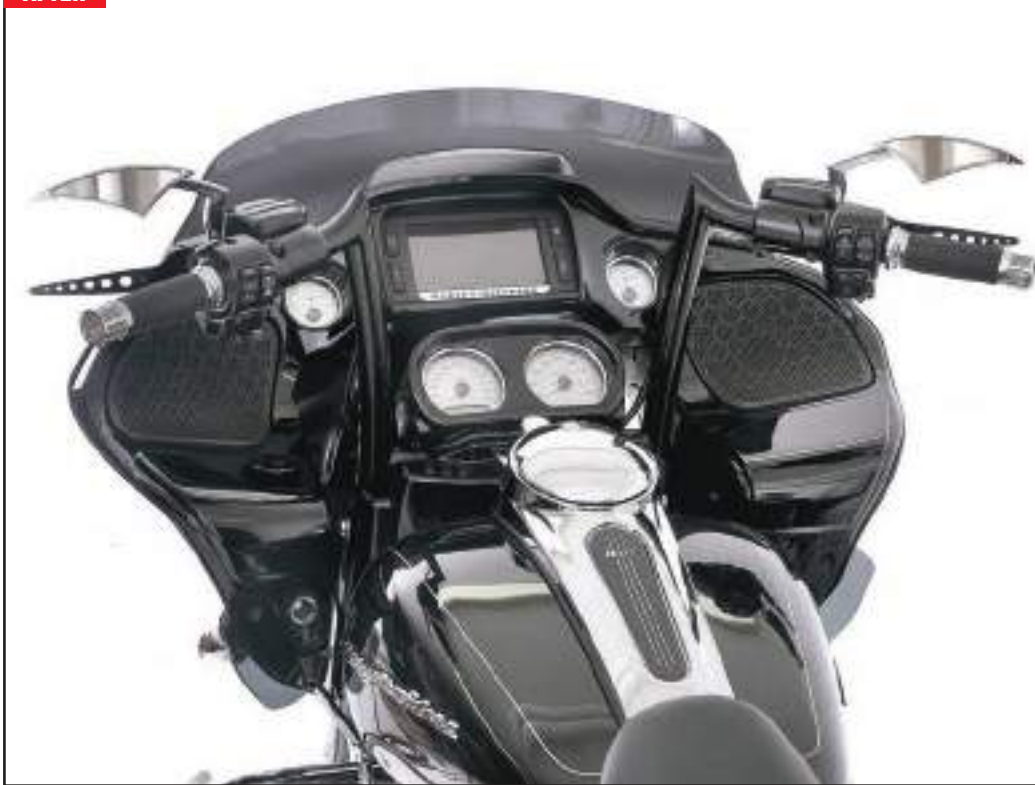
The 2016 Road Glide Special with Bagger Nation 10" OEM Monkey Bars, Power Mirrors, Racing Levers, Speed Freak Grips, and Super Riser Clamp installed.
