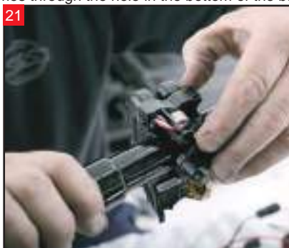
21 With the wiring ran through the handlebars, bring the switch assembly into position around the handlebars.
