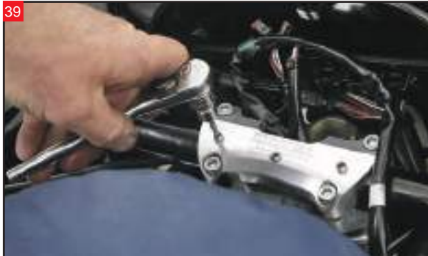
Tighten the three setscrews in the Super Riser Clamp in order to better secure the handlebars from movement.
