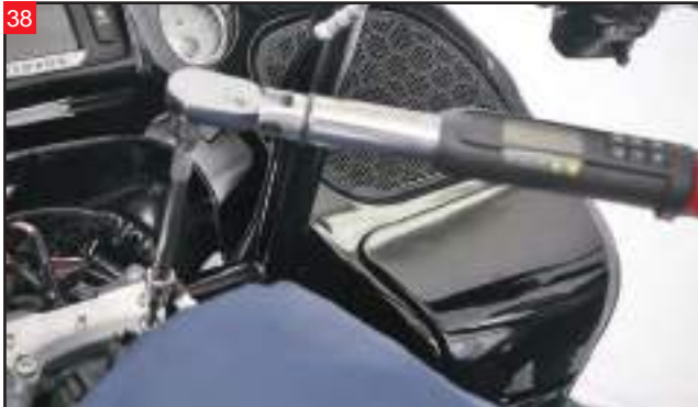
Evenly tighten down the top clamp bolts. Final torque of 16-20 foot/lbs.
