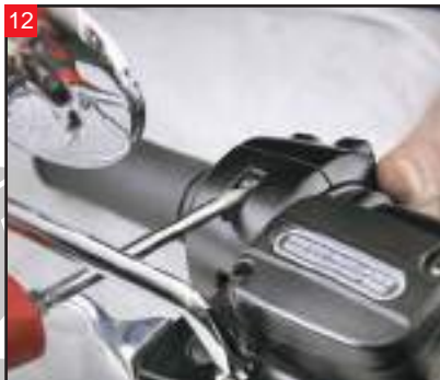
12 Use a T25 Torx to loosen the bolts holding the switch housings together.
