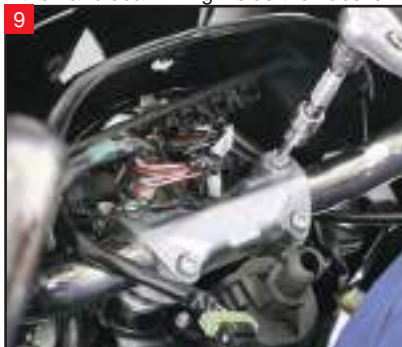
9 Loosen the four bolts holding the stock top clamp to the handlebar risers with a 1/4" Allen wrench. Maintain control of the handlebars while doing so.
