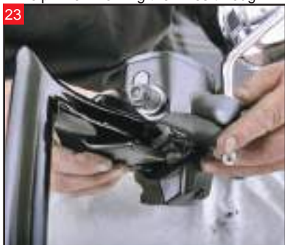
23 Bring the master cylinder and clamp in position next to the switch housing.
