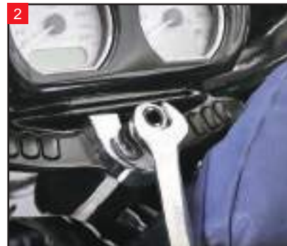
2 With a 7/8" wrench, remove the plastic nut from the ignition post. Lift the remaining pieces from the ignition post.
