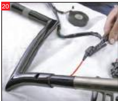
20 Gently feed the wiring through the openings in the handlebars. The hole at the bottom corner of the handlebars will help when working the wires through.
