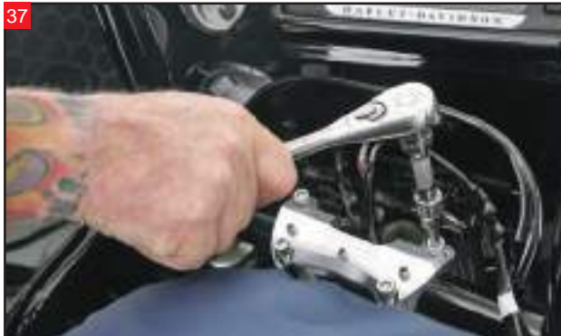
Apply blue thread locker to the stock top clamp riser bolts. Use these bolts when installing the Bagger Nation Super Riser Clamp.
