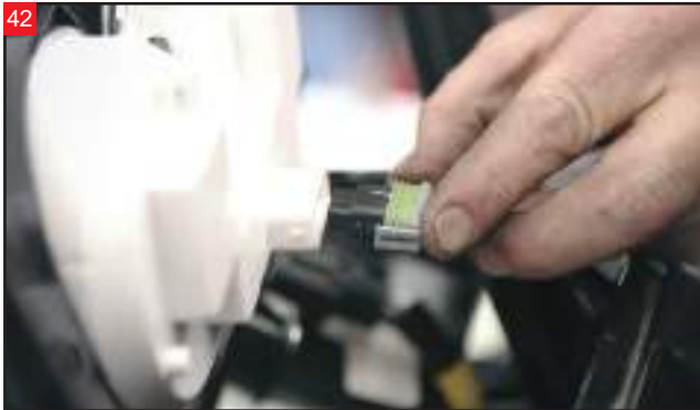
Bring the speedometer/tachometer housing into position. Plug in the wiring connector into the back of the gauge assembly.
