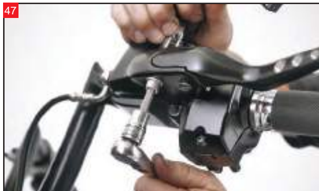
Position the Bagger Nation Power Mirrors in the stock mirror location. Use a 1/4" Allen to install the mirrors with the included bolts. Use blue thread locker on the hardware.
