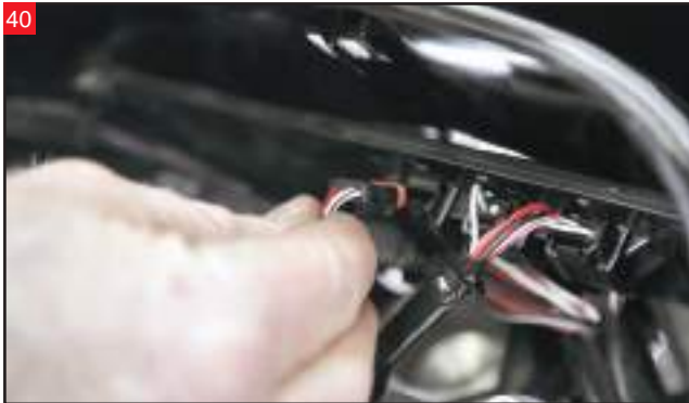
Reconnect the CANBUS wiring from the handlebar switch housings.
