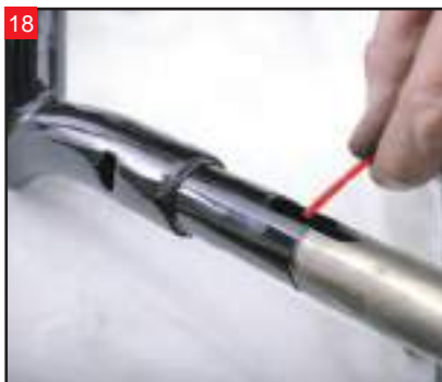
18 Feed the weed eater line through the top holes of the Bagger Nation Monkey Bars. Continue to work the weed eater line through the handlebars until it comes through the hole in the bottom of the bars.
