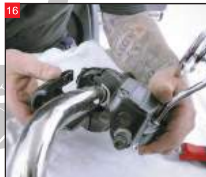
16 Repeat the process for the left side switch housing and clutch master cylinder.
