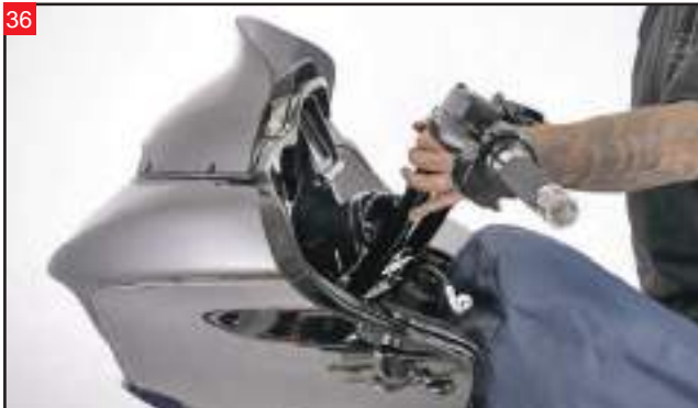
Bring the assembled handlebars back into position on the risers.
