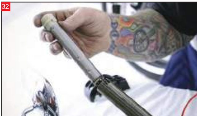
32 Repeat the process for the right side switch wiring, including the Twist Grip Sensor.
