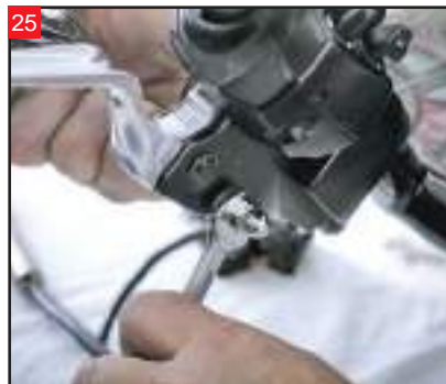
25 To remove the stock mirrors, loosen the acorn nut with a 1/2" wrench.
