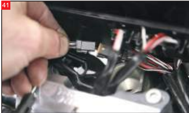
Plug in the connector for the Twist Grip Sensor.
