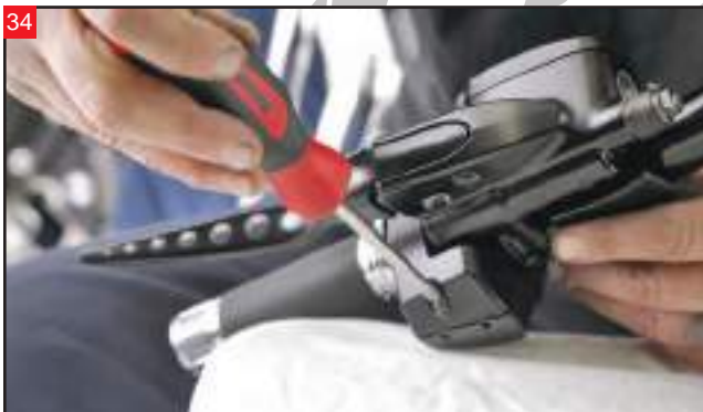
34 Use Torx drivers to tighten the hardware for the switch housing and front master cylinder.
