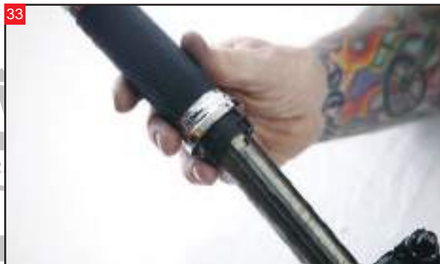
33 With the TGS installed in the handlebars, slide the right Speed Freak Grip over the end of the handlebar. Ensure the notches in the grip engage the notches in the TGS.
