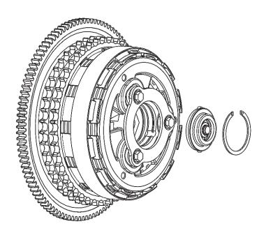
7. Using a 1 3/16" socket and an impact driver, remove the **right-hand thread** center clutch nut.
