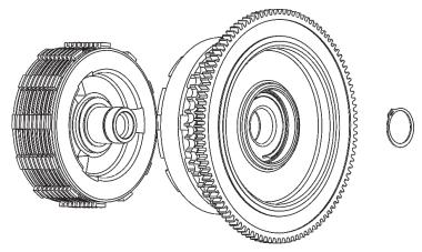
11. Using snap ring pliers, remove retaining ring from back of basket and press the bearing out of the basket.
