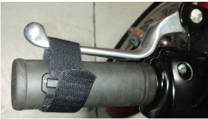
Clutch Lever Strap: to prevent unwanted launching.
