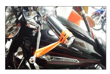
f) While still in **NEUTRAL**, quickly rev the engine between 3,000-5,000 RPM (1/4 to 1/2 throttle), then let it return to idle. Notice the movement in the clutch lever when the engine is revved. This is your Free Play Gain.
