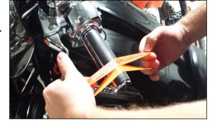
d) While holding the top end of the rubber band against the handlebar, stretch the band downward, then loop it through itself.
