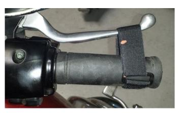
Brake Lever Strap: for use as a parking brake.
