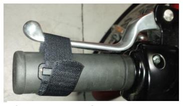
Clutch Lever Strap: to prevent unwanted launching.
