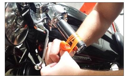
e) Pull the band through the loop, then attach it to the outside end of the clutch lever. This will take up the initial free play (slack) and put the lever in a position to detect the Free Play Gain.
