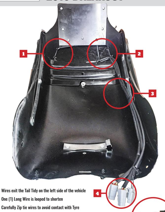
4 Three (3) Connector Plugs exit the front of the fender on the
