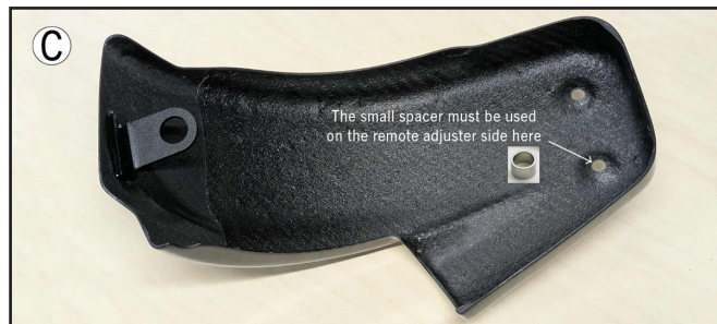
Softail models with Adjustable Preload Knob will use a small spacer (included) on the lower bolt hole
