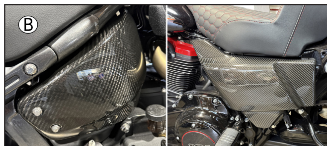
Softail models (left) will reuse stock hardware to install your new side covers. Touring models (right) simply press onto the frame same as stock.
