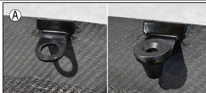
(Softail models only) The cone shaped rubber grommets on your original side covers must be transferred over to the new side covers.
