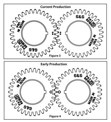
NOTE: Current production S&S Gear drive camshafts have timing marks shown in **Figure 3**. Older S&S gear drive camshafts, have the timing marks shown in **Figure 4** Cams with early and late gear styles must not be used together.
