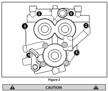
Failure to remove and install bolts according to correct procedure may result in parts damage not covered under warranty.
