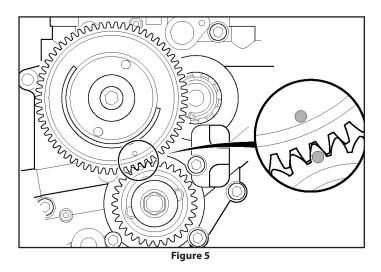
16. Place pinion gear on the pinion shaft with timing mark outward. Apply a drop of red thread locker to threads of 5/16"-18 x 3/4" Grade 8 crankshaft gear bolt, provided in S&S® Camshaft Installation Kit 106-5896 or obtained from another source. Apply a drop of clean engine oil under bolt flange. Using the washer removed in disassembly step G, install crankshaft gear bolt and tighten to 25 ft-lbs. torque.
