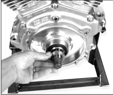
**CHARGING SYSTEM NOTE** - *If you are going to use a 45 amp alternator you must install a S&S® spacer (PN 31-4033). If you do not use this spacer the rotor could bottom out against the case when the sprocket shaft nut is tightened.*
