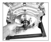
**CHARGING SYSTEM NOTE** - If you are going to use a 45 amp alternator you must install a S&S® spacer (PN 31-4033). If you do not use this spacer the rotor could bottom out against the case when the sprocket shaft nut is tightened.
