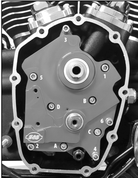
Picture 3: Cam Support Plate Screws (1-6) and Oil Pump Screws (A, B, C, D)
