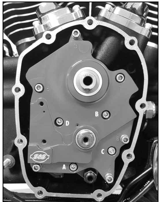
Picture 3b: Oil Pump Screws-Torque According to Step 22
