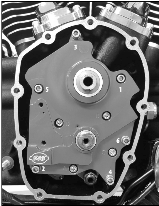
Picture 3a: Cam Plate Screws-Torque According to Step 32
