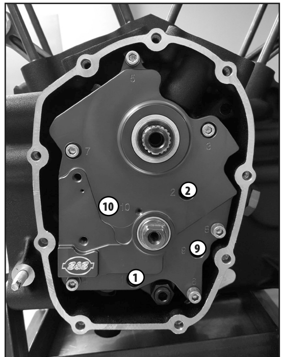
Picture 3b: Oil Pump Screws-Torque According to Step 23
