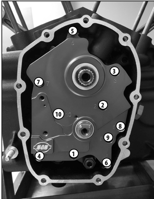
Picture 3: Cam Support Plate Screws (3-8) and Oil Pump Screws (1, 2, 9, 10)
