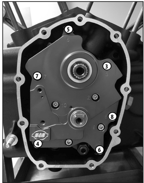
Picture 3a: Cam Plate Screws-Torque According to Step 21
