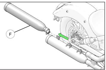
6. Remove lower muffler (G) by gently moving muffler up and down and side to side while sliding muffler assembly rearward.
