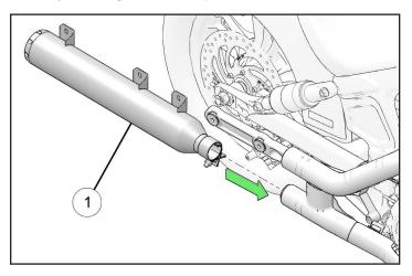
3. Install upper muffler onto rear head pipe assembly while loosely installing muffler clamp.
