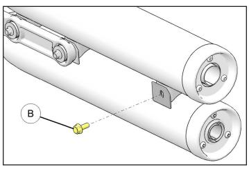
6. Make sure mufflers are properly aligned, torque bolts (B) and (C). Then torque nuts (A) on muffler clamps. Ensure clamp orientation is correct.
