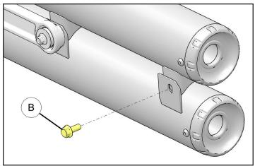
4. Remove two bolts  $\bigcirc$  washers  $\bigcirc$  (if installed) and exhaust isolators  $\bigcirc$  (if installed) connecting upper muffler to exhaust mount.
