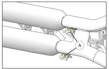
3. Remove bolt(B) at rear of exhaust assembly connecting upper and lower mufflers together.
