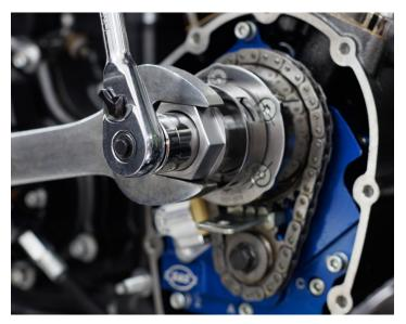
4. Remove the bolt while holding the tool in place.
