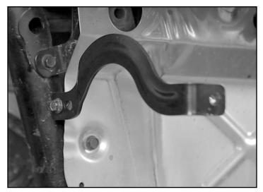
7. Install the muffler mounting studs into the rubber isolators on the
