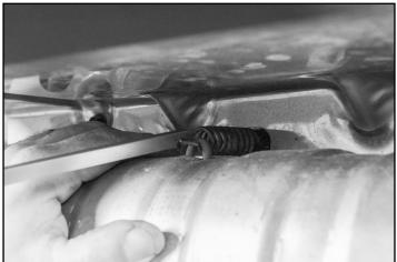
3. Remove the 3 nuts from the header pipe
