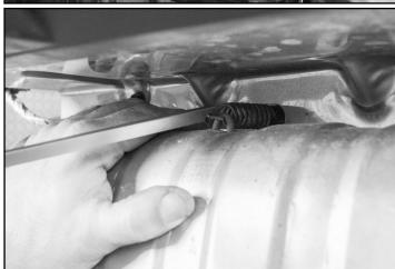
10. Install the rear plastic muffler cover. (4 Torx headed fasteners)
