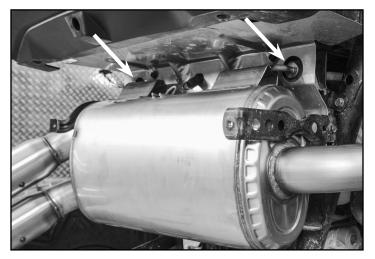
8. Install a new flange gasket if needed. Put a dab of high temp antiseize on the studs and install the three nuts on flanges. Torque nuts to 18 ft-lb (24 Nm)
