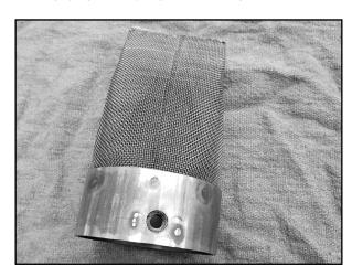
**NOTES:** A plugged spark arrestor will cause performance loss. Always replace a cracked or damaged spark arrestor before operating.
