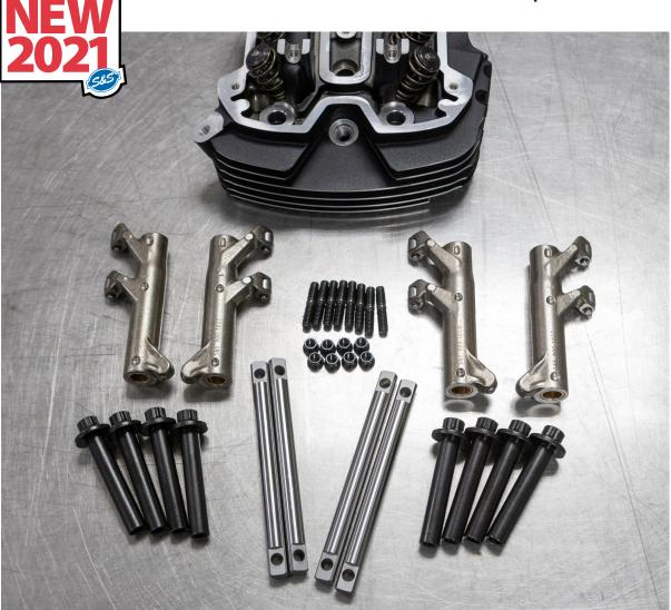
M8 Rocker Arm Shafts are a direct replacement for OEM units. Replace stock or broken OEM pieces with proven S&S Performance parts that are **66% stronger than stock!**
