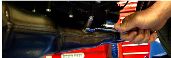
3. Loosen head pipe hardware.
