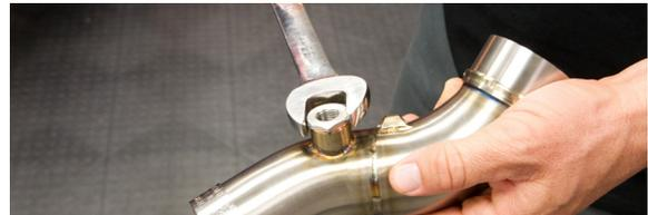
10. Apply thin layer of anti-seize to slip-tube and attach to muffler using supplied hook springs.
