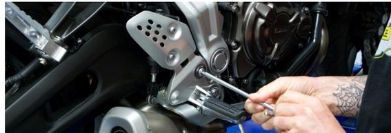
5. Remove muffler mounting bolts.
