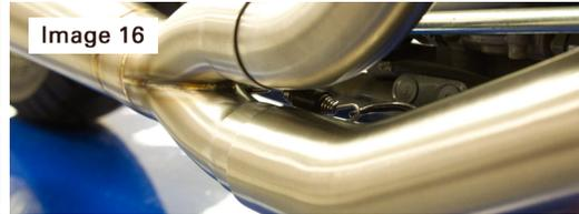
15. Install and tighten muffler mounting flange bolts 5/16" x 3/4".
