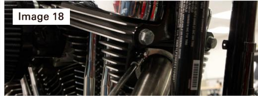
17. Feed clamps through head shield retainers. Install heat shields onto header pipes and tighten clamps.
