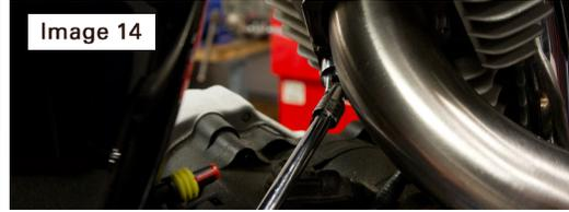
14. Install clip nuts onto muffler and install muffler onto head pipes. Attach with supplied hook springs.
