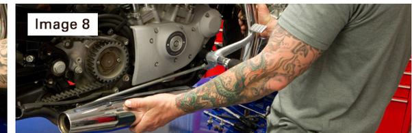
8. Remove bolt from rear end of brake rod bolt to gain access for next step. (Reference image 9)
