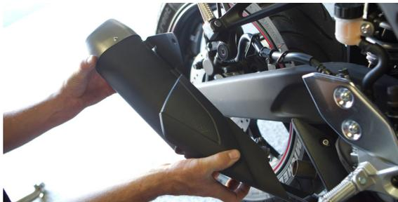
3. Attach TBR muffler to TBR slip tube using springs provided.
