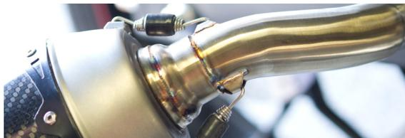
4. Loosely install supplied join clamp to slip tube.
