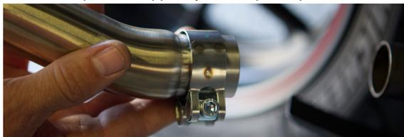
5. Install TBR muffler assembly using OEM hardware and supplied rubber lined muffler clamp.
