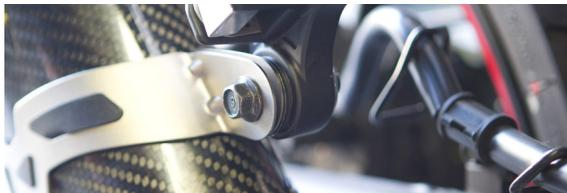
6. Tighten joint clamp and muffler strap.
